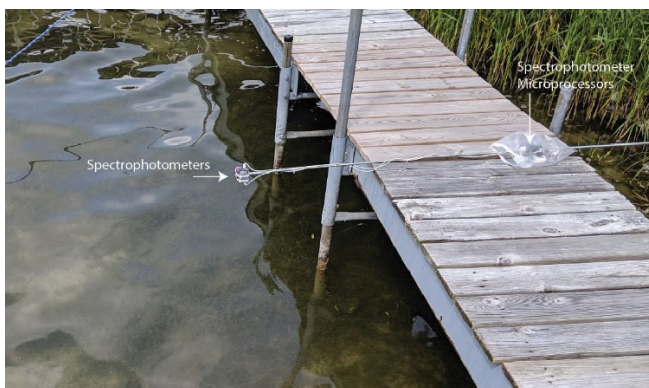
Fig. 3. The spectrophotometer in the field.
