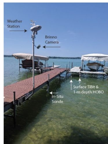
Fig. 4. A weather station, automated camera and water sensors at a dock site.
